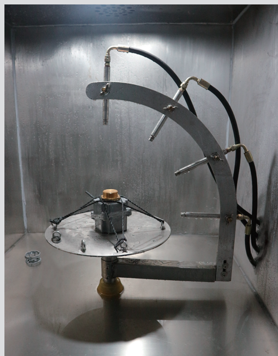
Enclosure during IPx9K test
