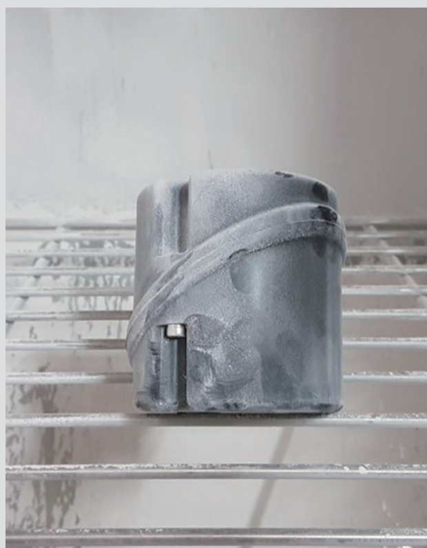
Enclosure during IP6x test
