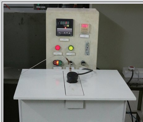
Sodium hypochloride test bath
