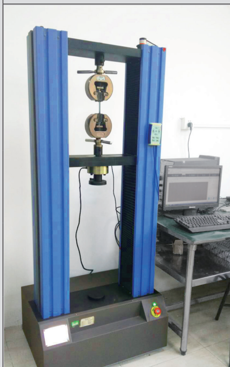
Tensile strength at break measurement equipment
