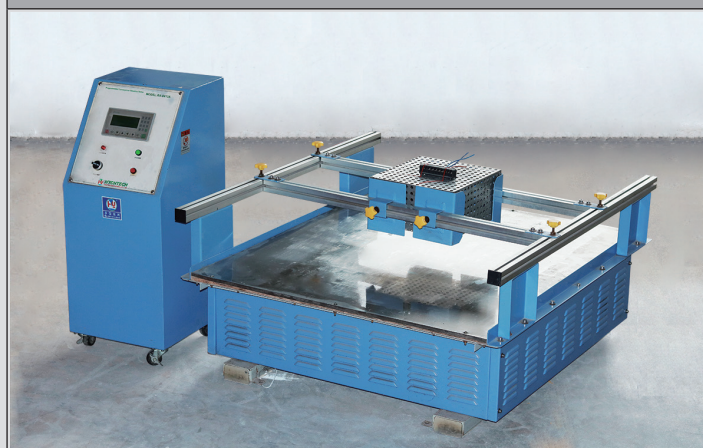
Vibration test equipment
